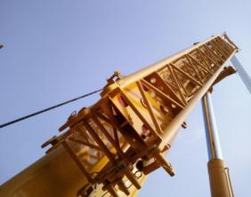
**副起重臂:** Jib: ■两节桁架式副起重臂 ■Two-section lattice jib
